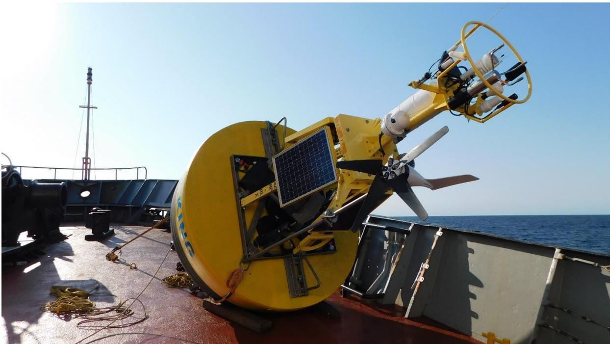
**Figure 3.** Image of the AZMP-HLX Viking Buoy positioned on the foredeck of CCGS *Hudson* prior to its deployment during the HUD2021185 mission. Due to a lack of ballast, the buoy automatically shifts to a horizontal position when lifted. *Picture contributed by Diana Cardoso.*
