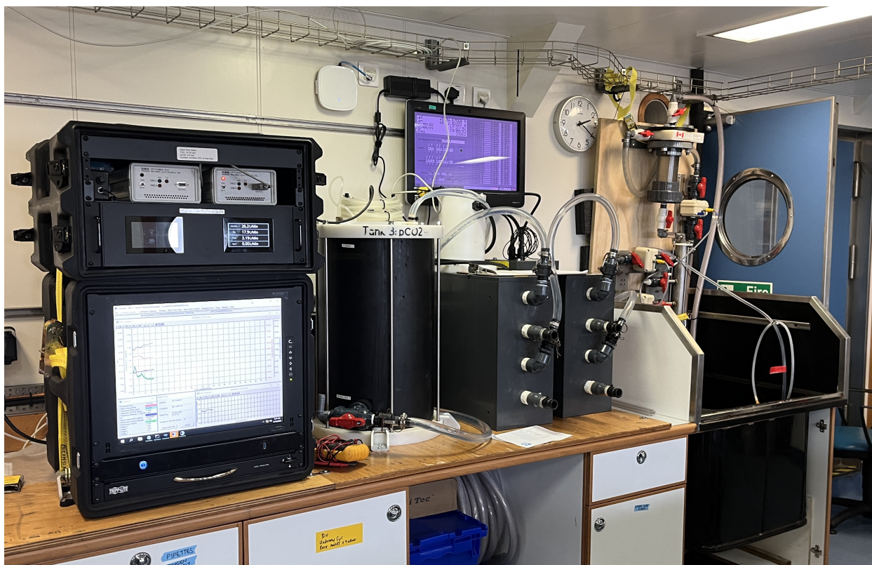
Figure 7: BIO Underway system installed on a bench in the General Purpose Lab on board the RRS Discovery during the DY16902 mission.
