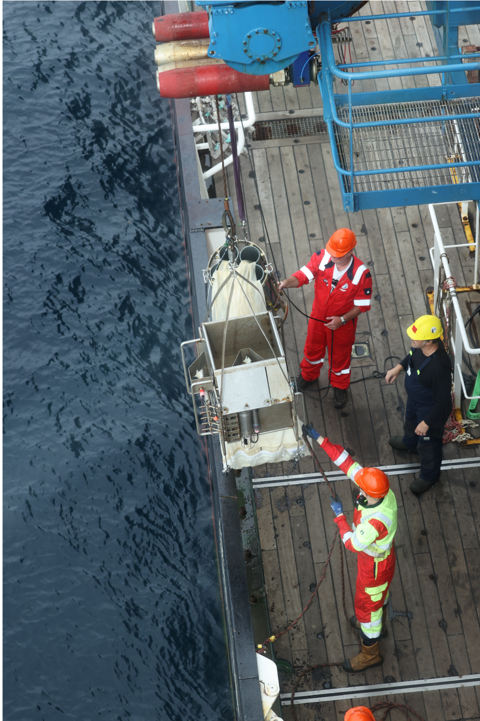
Figure 4: Multinet sampling system used to collect stratified zooplankton samples during the DY16902 mission. An auxiliary winch on the bullhorn boom was used to lift the cod end over the rail.
