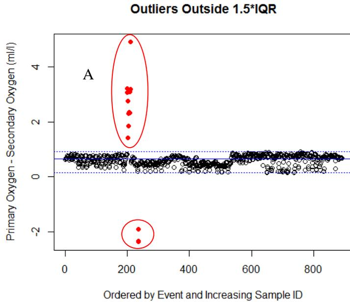
**Figure 4.** The difference between primary oxygen sensor #0133 and secondary oxygen sensor #0042. Outliers in red were removed prior to proceeding with Soc calculation: **A**) outliers from Event 44 (BBL\_07 : 440470-440478), and **B**) Event 48 (HL\_07: 440502 - 440504). The mean difference between sensors before outlier removal (solid blue line) is 0.65 ml/l. The lower and upper dotted blue lines are 0.14 and 0.90 ml/l respectively.
