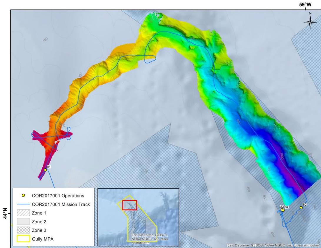
**Figure 25.** The multibeam survey of the Gully MPA. Note the sound velocity profiles conducted at the beginning (Event 81) and end (Event 82) of the survey. Events 83 and 84 are the CTD and net profile at GULD\_03.
