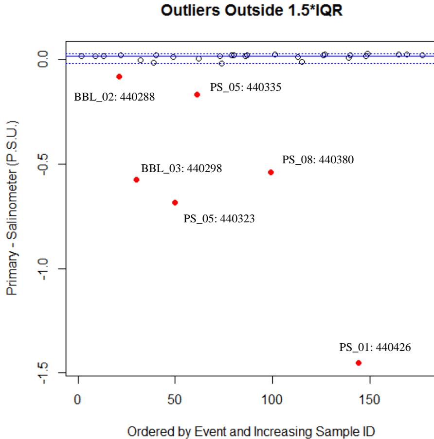
**Figure 11.** The difference between the primary sensor (#3562) and the salinometer after the removal of erroneous sensor data prior to event 45. Six erroneous values were removed prior to proceeding. The mean difference (solid blue line) between the primary and salinometer was  $1.58e-02$  and the IQR upper limit is  $2.53e-02$  and the lower limit is  $-2.11e-02$  (dotted blue lines).
