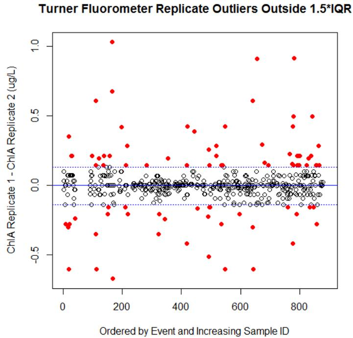
**Figure 18.** The outlier Turner replicates removed prior to determining the relationship between the Turner Fluorometer values and the SeaPoint sensor values collected during the COR2017001 mission. The mean difference is 0  $\mu\text{g/L}$ , the upper limit of 1.5\* IQR is 1.29  $\mu\text{g/L}$  and the lower limit is -1.41  $\mu\text{g/L}$ .
