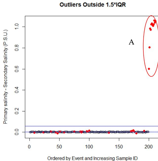
**Figure 10.** A) when the plumbing for both sensors was blocked during event 44 at BBL\_07 (440467 to 440478). The mean difference (solid blue line skewed by the inclusion of event 44) is 5.784e-02 and the IQR upper limit is 6.5e-03 and the lower limit is -5.0e-04 (dotted blue lines).
