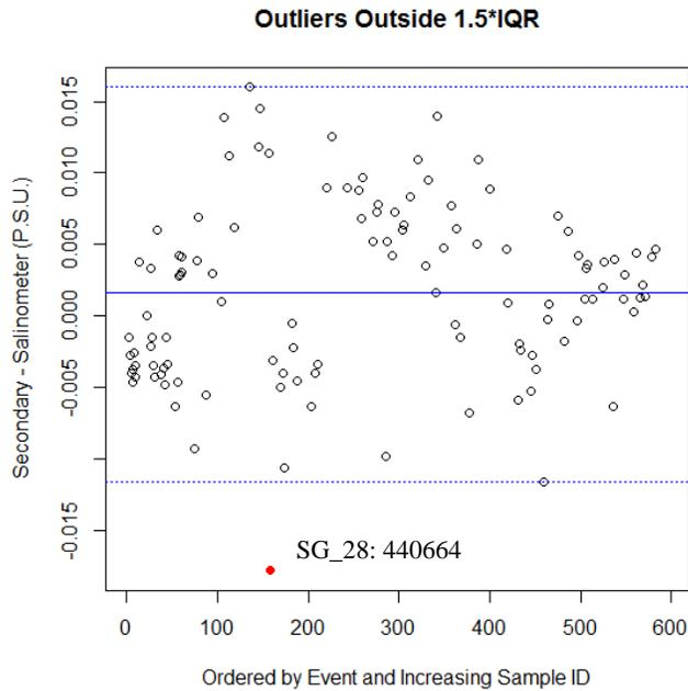
**Figure 16.** The difference between the secondary sensor (#1076) and the salinometer after the removal of erroneous sensor data after event 44. Four erroneous values were removed prior to proceeding. The mean difference (solid blue line) between the primary and salinometer was  $1.6 \times 10^{-3}$  and the IQR upper limit is  $1.60 \times 10^{-2}$  and the lower limit is  $-1.16 \times 10^{-2}$  (dotted blue lines).
