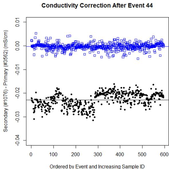
**Figure 17.** Before correction with new coefficients (black dots), the average difference between secondary (#1076) and primary (#3562) conductivity was  $-2.2833 \times 10^{-2}$  mS/cm (solid black line). After correction, the average difference between sensors was  $-2.9730 \times 10^{-4}$ .
