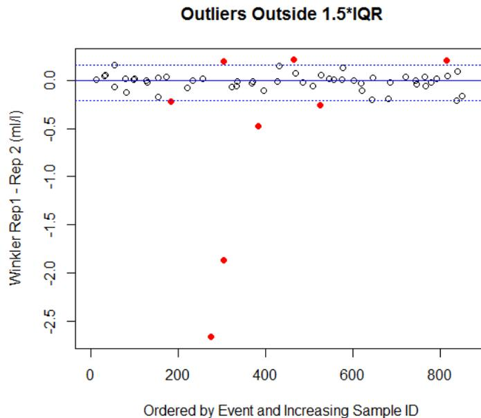
**Figure 5.** The mean difference (solid blue line) between 1<sup>st</sup> and 2<sup>nd</sup> Winkler replicates (-0.003 ml/l). The lower and upper dotted blue lines are -0.21 and 0.16 ml/l respectively. Note the 8 outliers in red that were removed prior to proceeding with Soc calculation (sample ID numbers 440452, 440557, 440586, 440587, 440667, 440748, 440807, and 441096).
