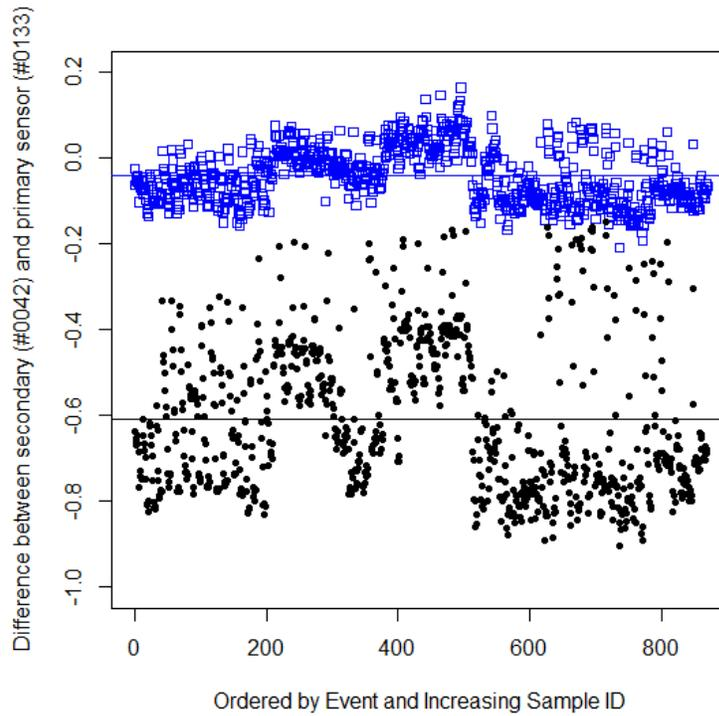
**Figure 8. A)** Black dots – uncorrected difference between outlier free secondary sensor values (#0042) and primary sensor (#0133) values (black line is the mean = -0.61 ml/l). Blue squares – Soc corrected difference between secondary sensor (#0042) values and primary sensor (#0133) values (blue line is the mean= -0.0410 ml/l).
