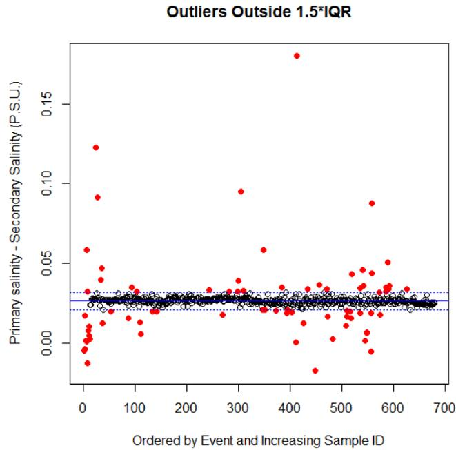
**Figure 14.** The mean difference between the primary and secondary sensors after event 44 is  $2.66 \times 10^{-2}$  (solid blue line), the IQR upper limit is  $3.16 \times 10^{-3}$  and the lower limit is  $-2.10 \times 10^{-2}$  (dotted blue lines).
