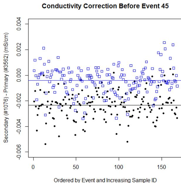
**Figure 13.** Before correction with new coefficients (black dots), the average difference between secondary (#1076) and primary (#3562) conductivity was  $\sim 2.3259 \times 10^{-3}$  mS/cm (solid black line). After correction, the average difference between sensors was  $4.1477 \times 10^{-4}$ .
