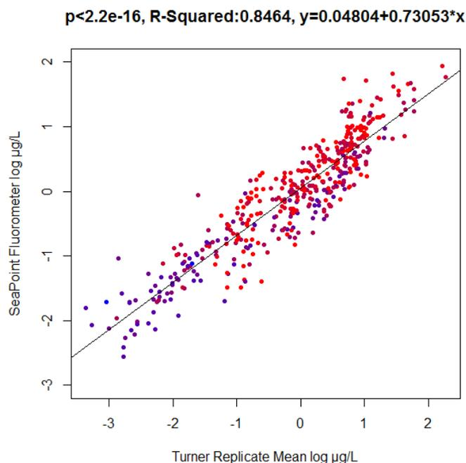
**Figure 20.** The log/log plot of SeaPoint Fluorometer values and the corresponding mean replicate Turner Fluorometer values colour coded by depth, where red and dark red are shallow (closer to the surface) and purple and blue are deep (closer to 100 m).
