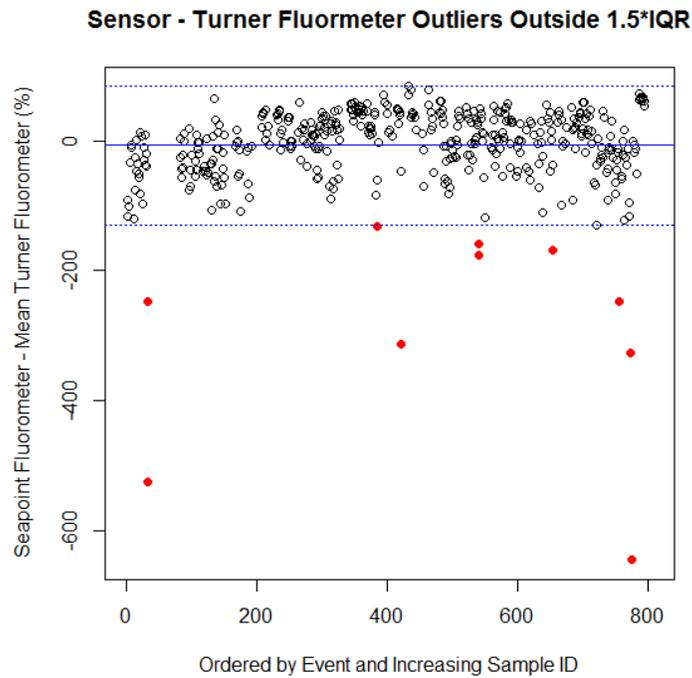
**Figure 19.** The outliers identified from calculating the % difference between Turner Fluorometer values and the SeaPoint sensor values collected during the COR2017001 mission.
