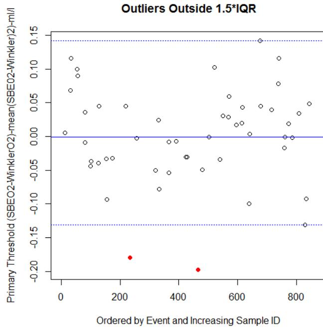
**Figure 6.** Outlier “threshold” values for the primary sensor were removed. **A)** - Event 97 at LL\_08: 440752 and, **B)** Event 53 at HL\_06.7: 440517. The solid blue line is the mean value of the primary sensor threshold (~0 ml/l) and the lower and upper dotted blue lines are -0.13 and 0.14 ml/l respectively. These outlier data points were removed and the remaining data were used to calculate the primary Soc values.
