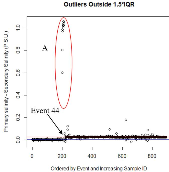
**Figure 9.** A) when the plumbing for both sensors was blocked during event 44 at BBL\_07 (440467 to 440478). The mean sensor difference prior to event 44 was 0.00294 P.S.U (blue line) and the difference after event 44 was 0.02663 P.S.U. (red line).
