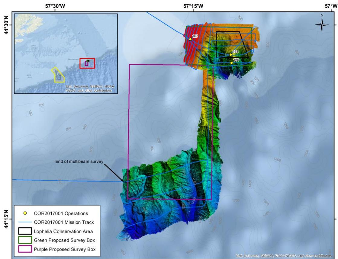
**Figure 26.** The multibeam survey of the Stone Fence Lophelia Conservation Area. The Green box proposed by OCMD encompassed the entire closure area. The purple box was only partially complete before the vessel was required to begin the steam to Halifax. The survey was started at event 167, 2 SVPs were conducted (events 168 and 169) and the survey was ended where noted in the figure.
