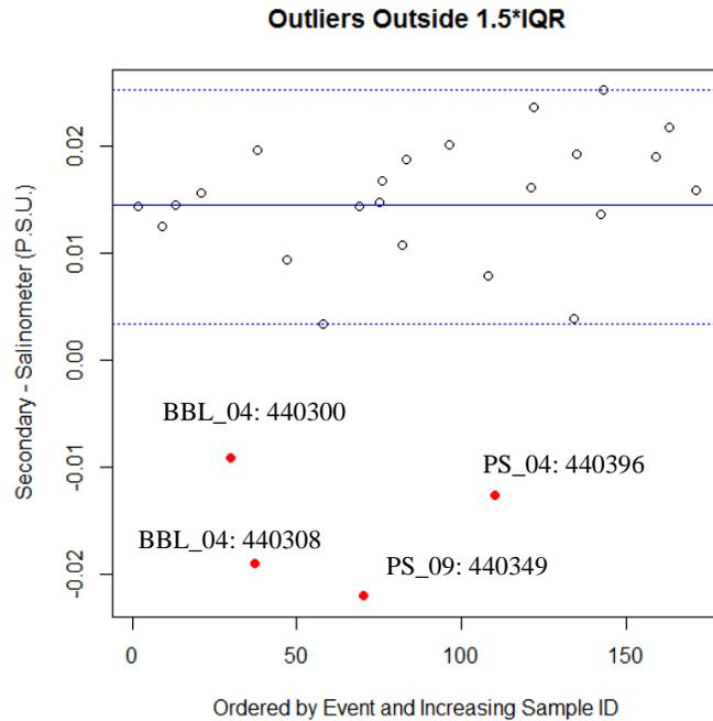
**Figure 12.** The difference between the secondary sensor (#1076) and the salinometer after the removal of erroneous sensor data prior to event 45. Four erroneous values were removed prior to proceeding. The mean difference (solid blue line) between the primary and salinometer was  $1.45 \times 10^{-2}$  and the IQR upper limit is  $2.52 \times 10^{-2}$  and the lower limit is  $3.30 \times 10^{-3}$  (dotted blue lines).
