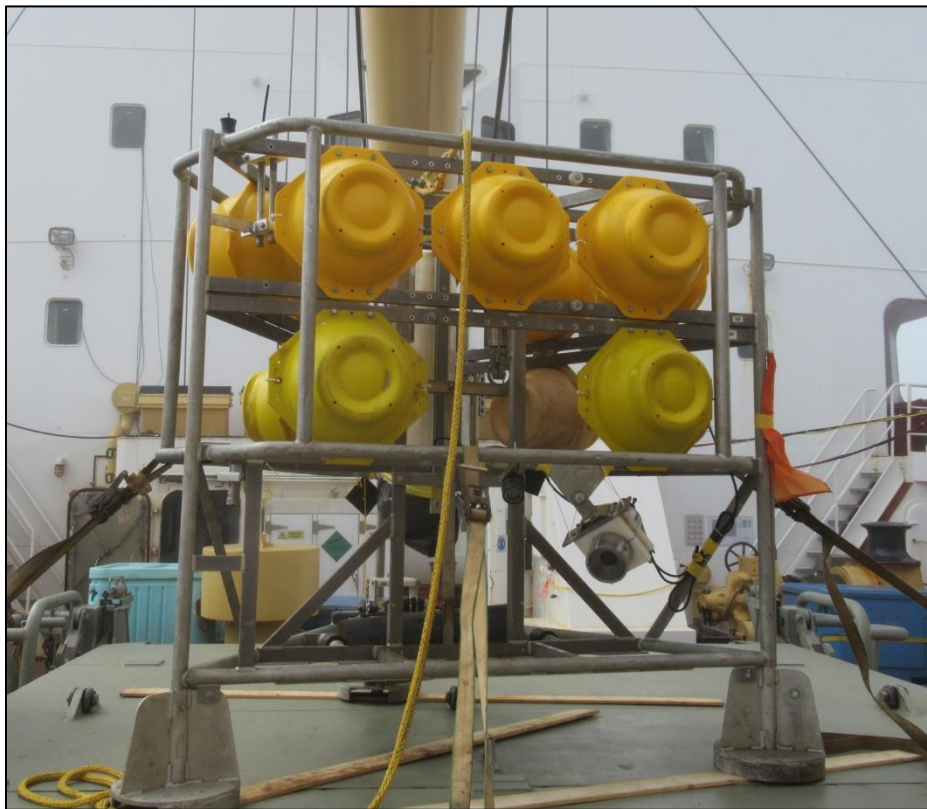
Figure 9. Benthic lander owned by NIOZ. Shown situated on the cargo hold doors, where it was temporarily secured prior to deployment. Photo credit DFO.
