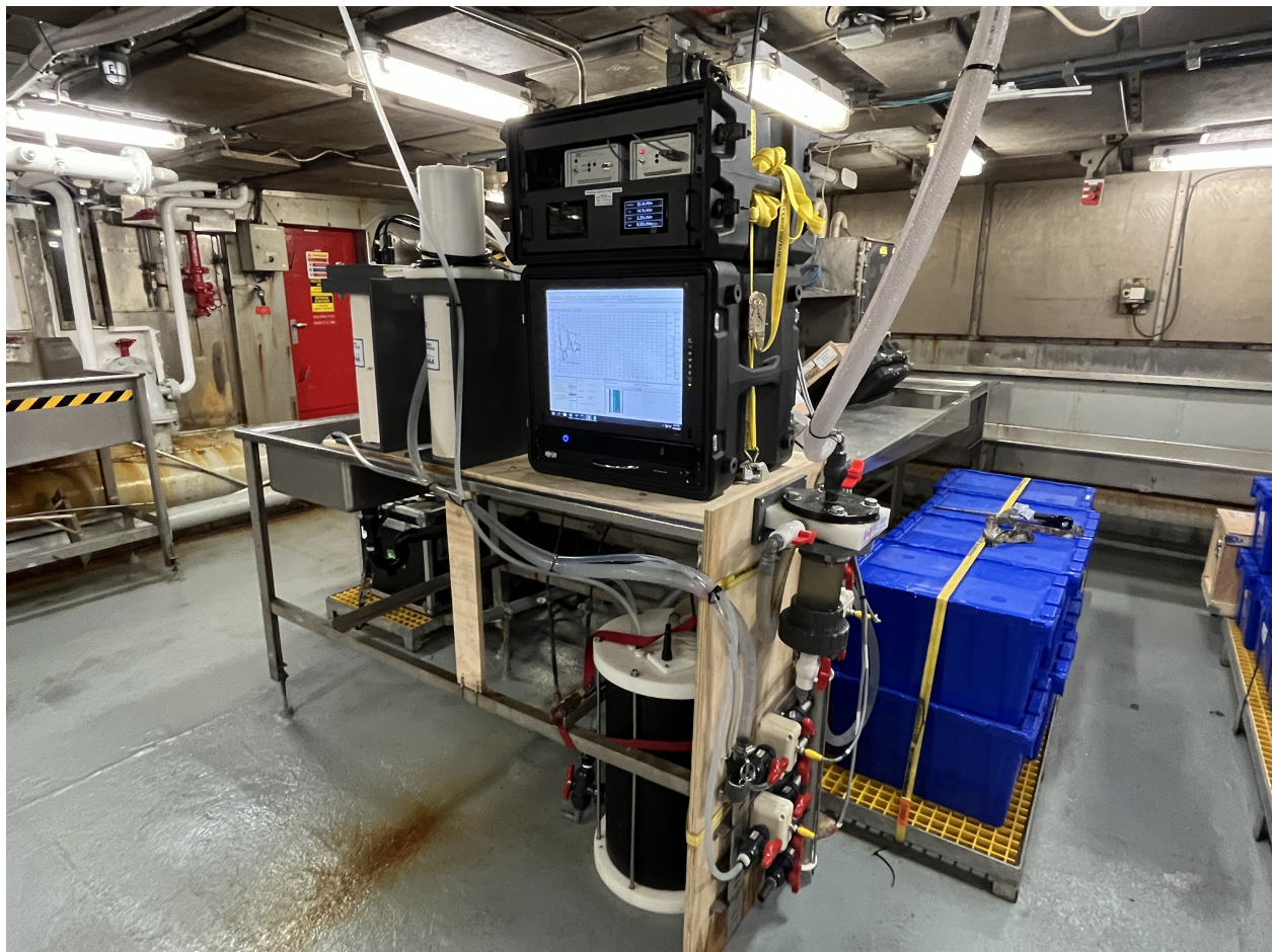
Figure 5. The BIO Underway system installed on a bench in the Wet Lab on board the CCGS Teleost during the 2024 spring AZMP survey (TEL2024880).
